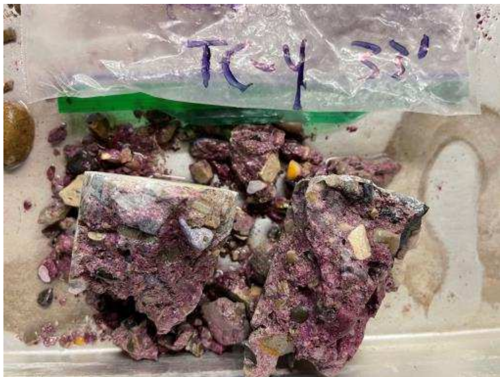
Photo 4: Broken surfaces of Core TC-4 (33') after application of phenolphthalein stain. Areas not stained magenta are carbonated. No Carbonation apparent.
