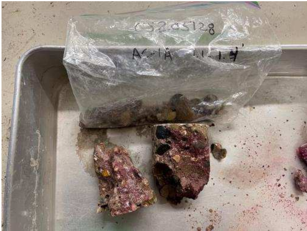
Photo 1: Broken surfaces of Core AC-1A (1.1'-1.4') after application of phenolphthalein stain. Areas not stained magenta are carbonated. No Carbonation apparent.
