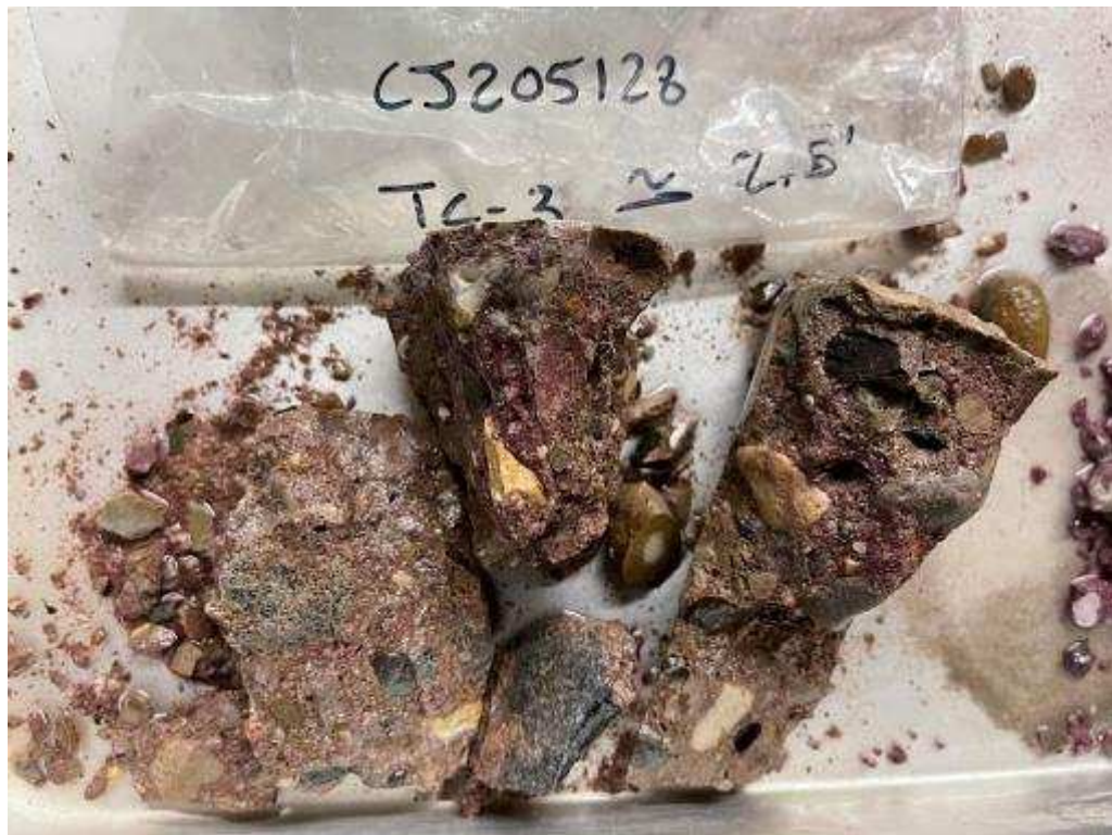
Photo 3: Broken surfaces of Core TC-3 (2.5') after application of phenolphthalein stain. Areas not stained magenta are carbonated. No Carbonation apparent.
