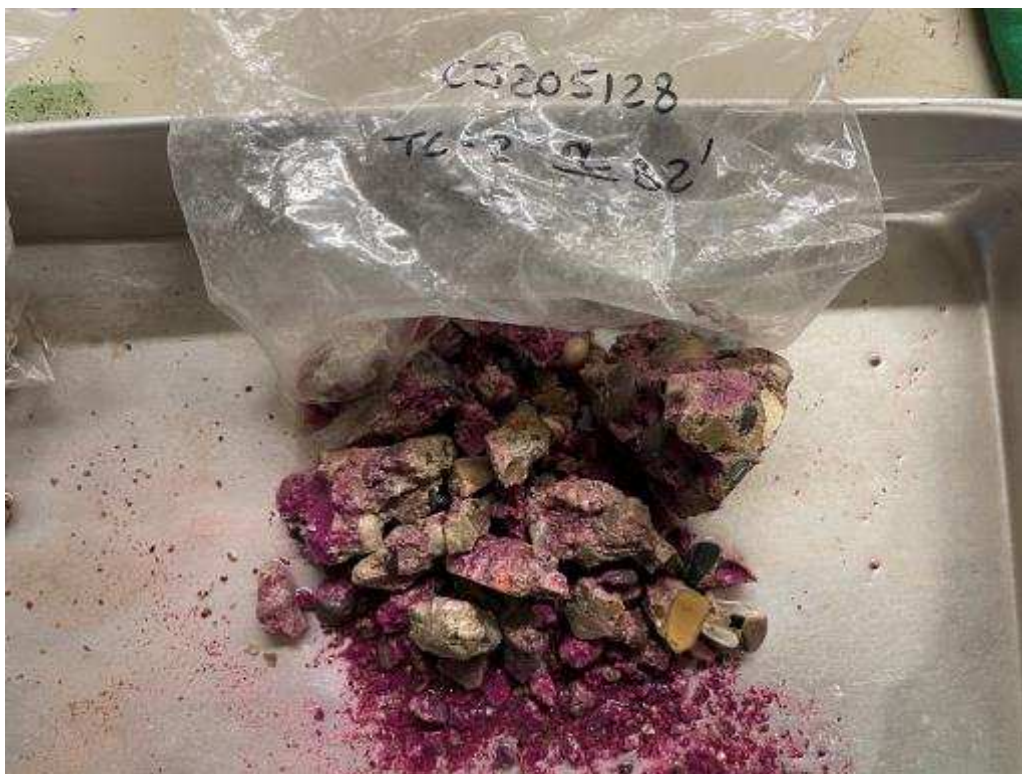
Photo 2: Broken surfaces of Core TC-2 (32') after application of phenolphthalein stain. Areas not stained magenta are carbonated. No Carbonation apparent.
